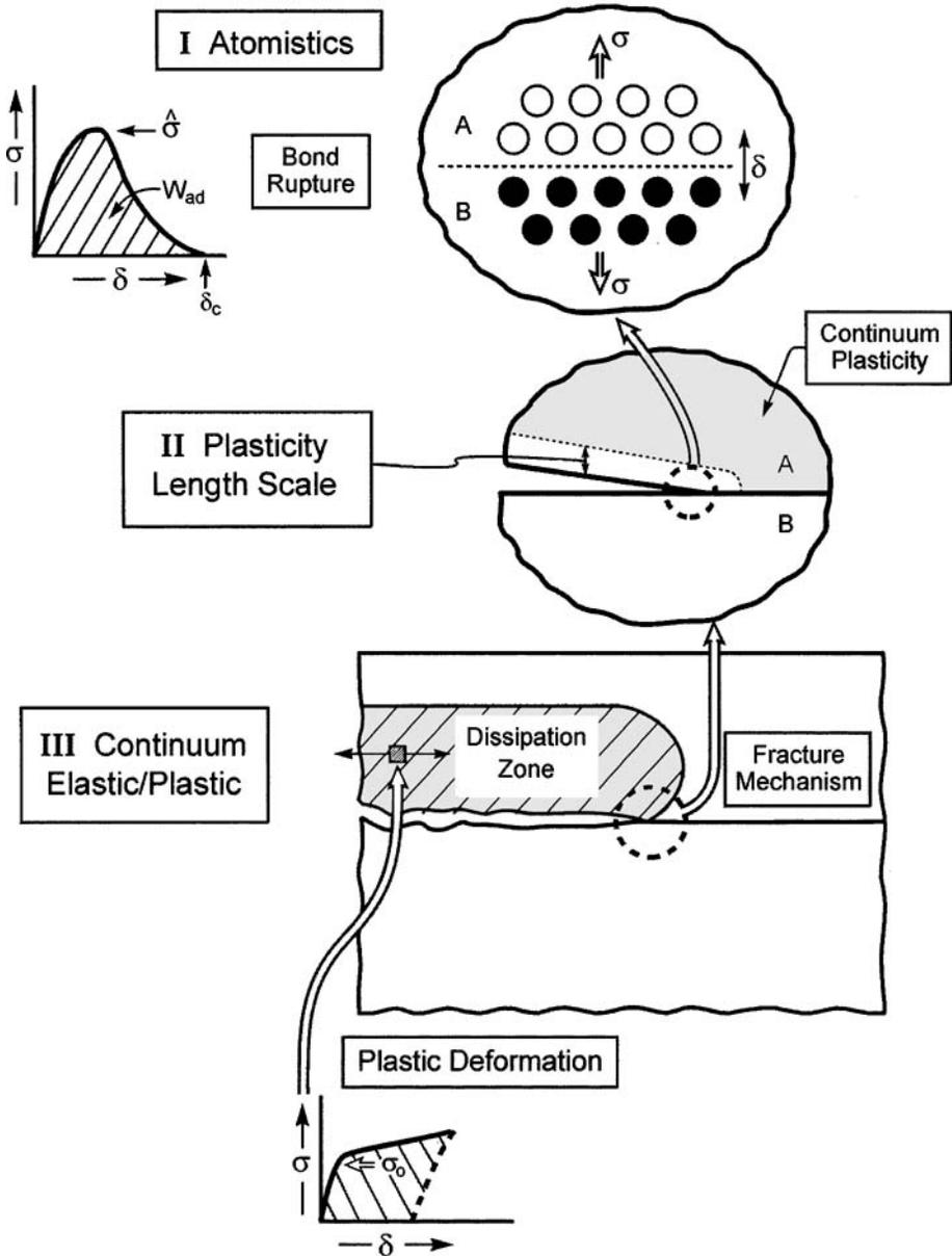
**Figure 6.** A schematic illustrating the zones of inelastic deformation that occur around interface cracks, with associated length scales.
