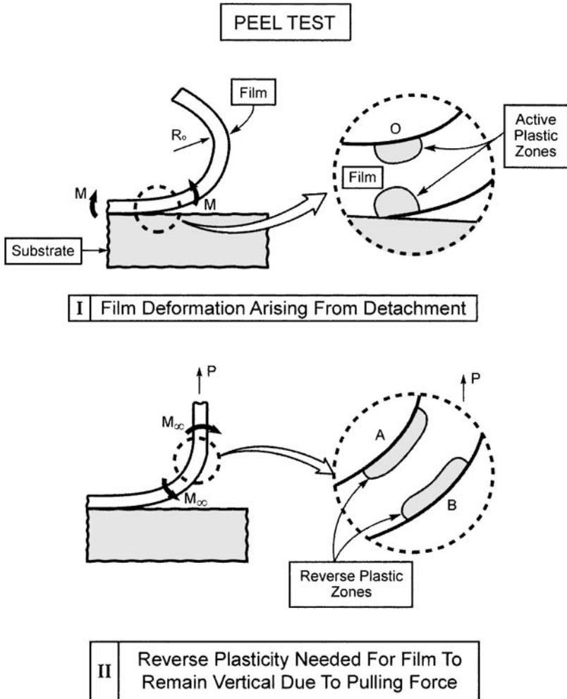
**Figure 3.** The peel test with a schematic indicating the plastic zones that arise because of bending (near-tip and reverse), which complicate interpretation of the measurements. In step I, film curvature arises because of the moment  $M$  near the tip that causes delamination, with consequent plasticity. In step II, the straightening of the film required by the applied loading is demonstrated, along with the zones of reverse yielding.
