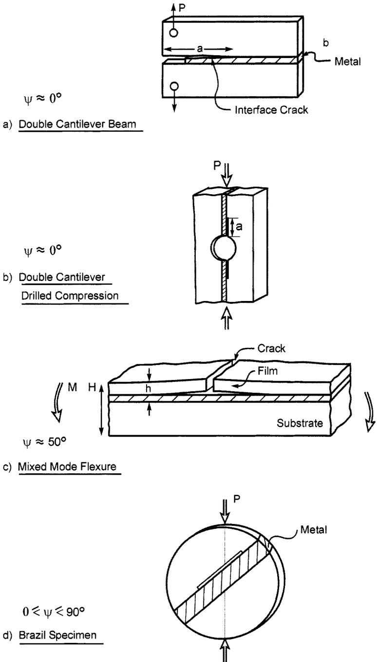
**Figure 2.** Test configurations used to measure the interface toughness on bonded bi-material systems.
