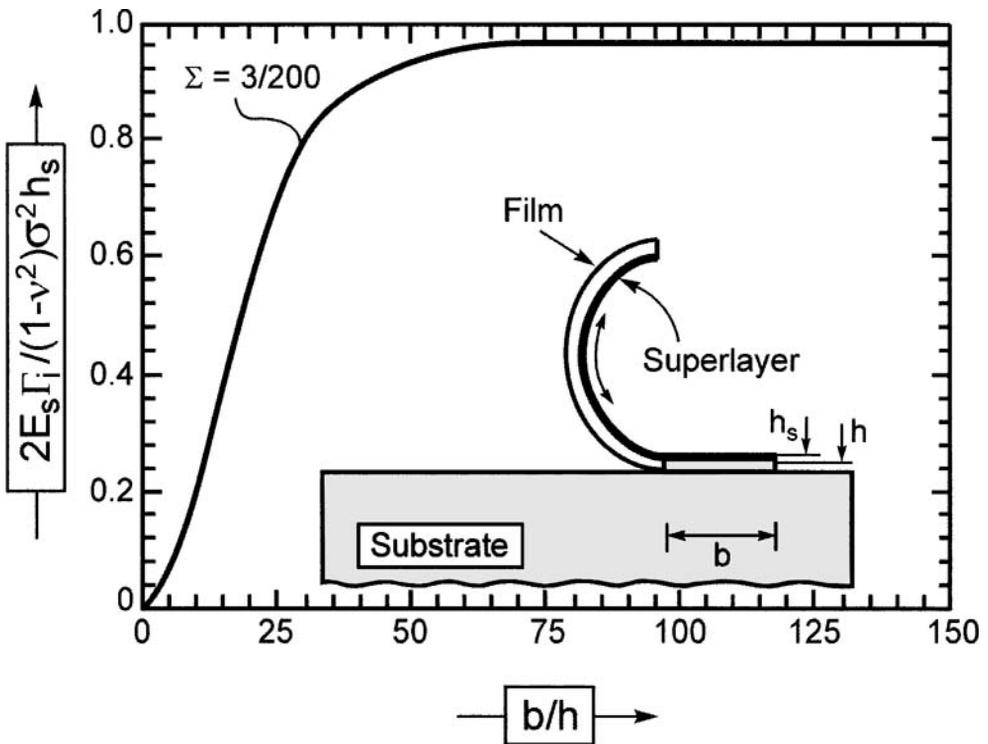
**Figure 5.** Superlayer method for measuring the interface adhesion between thin films and brittle substrates. Also shown is the energy release rate as a function of the length of the remnant ligament.
