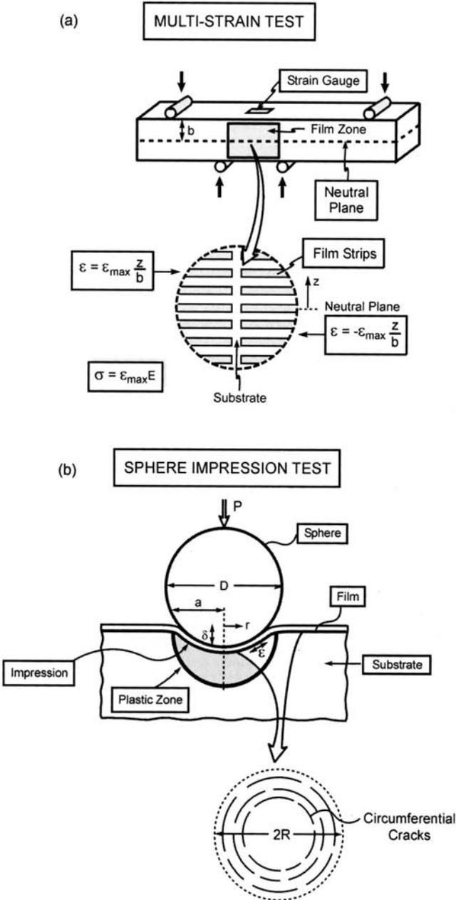
**Figure 4.** Tests used to measure the toughness of interfaces between thin films and a ductile substrate: (a) multi-strain test, (b) sphere impression test.
