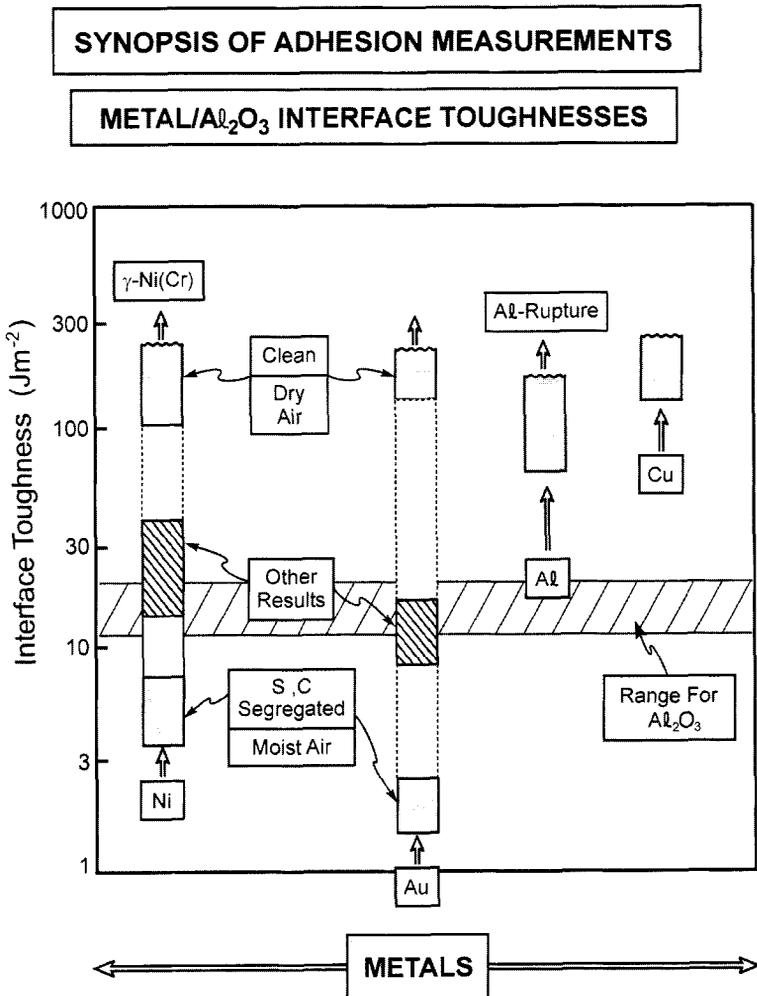
**Figure 1.** The range of toughness found between various metals and  $Al_2O_3$ . Note that many results reside in discrete domains that depend on "cleanliness".
