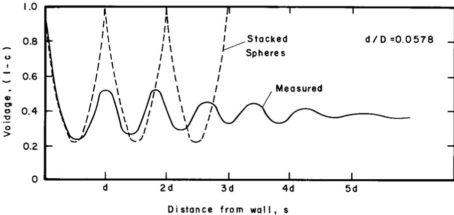
Figure 1-5. Voidage ( $1 - c$ ) as a function of distance from the pipe wall. (Data from Ridgeway and Tarbuck, 1968.)
