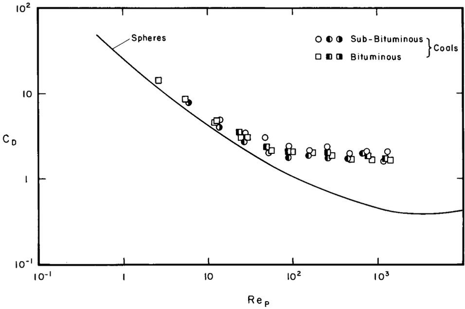
Figure 1-6. Particle drag coefficients for coals.
