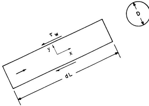
Figure 1-2. An elemental control volume for a pipeline.
