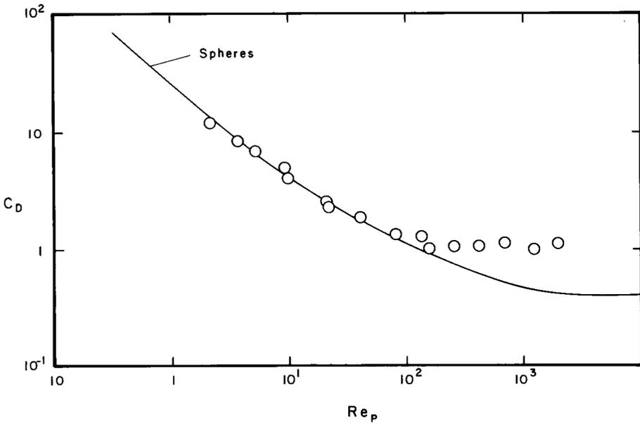
Figure 1-7. Particle drag coefficients for sands and gravels.
