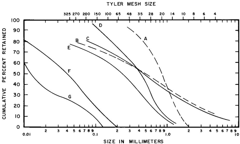
Figure 1-3. Some typical particle size distributions: A: Rosin-Rammler,  $m = 2$ ; B: Rosin-Rammler,  $m = 0.5$ ; C: -50 mm washed coal; D: potash (KCl) mill slurry; E: "long distance pipeline" coal slurry; F: boiler feed coal slurry; G: copper ore flotation cell underflow.
