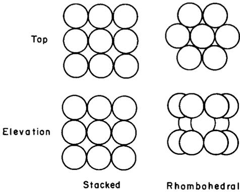
Figure 1-4. Two particle packing arrangements.
